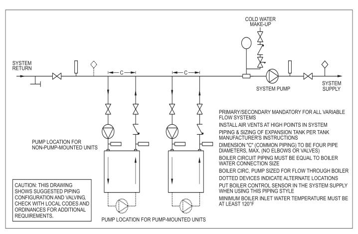
Figure 6. Hydronic Piping — Multiple Boilers, Primary Secondary System.
